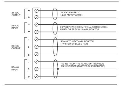
The 24 VDC field wiring needs to be of an appropriate gauge for the number of annunciators and the total wiring run length. Use the *Current Drain for Battery Calculations* on page 5 to calculate the maximum current for all annunciators summed together.
